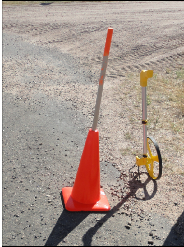
Figure 6 - Sight Distance Rods and Measuring Wheel
